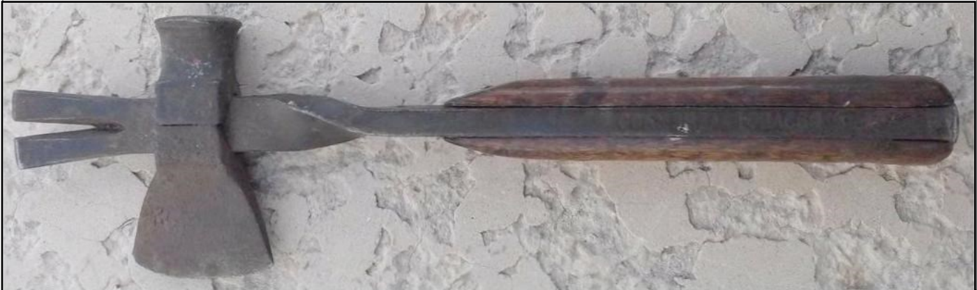
HT-13 12 1/2" Box Opener One End, Blade, Hammer, Metal Handle has Advertising "Cornbread Tobacco" on Edge Between Wood Grips
