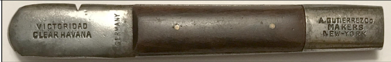
SEP-07 5 5/8" Notched Blade, Bar w/ Wood Insert Handle, Indented Printing
