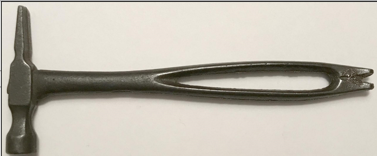
SHM-19 6 3/4" to 7 1/4" Notch At Blade, Hollow Handle, Hammerhead w/ Pointed Peen
