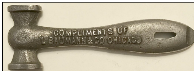
DHM-17 5" No Notch in Stepped-Down Blade End, Nail Puller in Handle, Raised Printing
