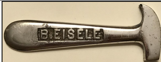
SHM-27 3 3/4" Small Hammer, Claw, Rounded Head, Wider Blade, Raised Printing
