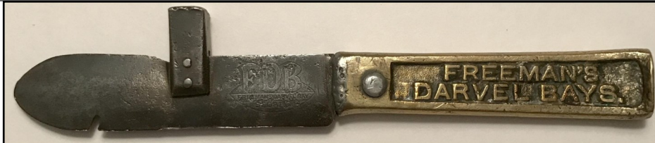
SEP-26 7 1/2" Long Notched Blade, Hammer, Brass Handle, Raised Printing
