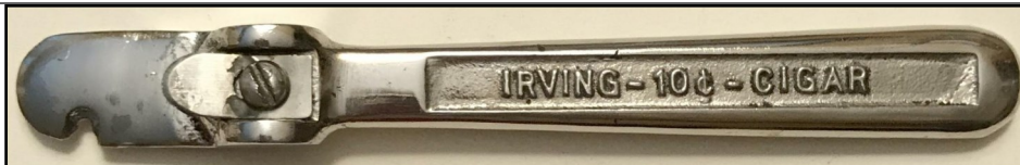
DHM-16 5 1/8" Notched Blade, Guide Along Double Hammers to Prevent Blade From Entering to Far Into Cigar Box, Raised Printing in Bossed Area (Appeared in 1907 Brunhoff Catalog)
