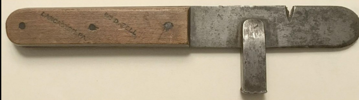
SEP-37 6 7/8" Long Notched Blade, Square Hammer, Wood Handle, Indented Printing
