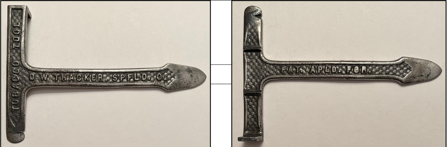
MIS-28 6 3/4" Notched Blade, Flat Hammer, Pry-Bar End, Raised Printing
