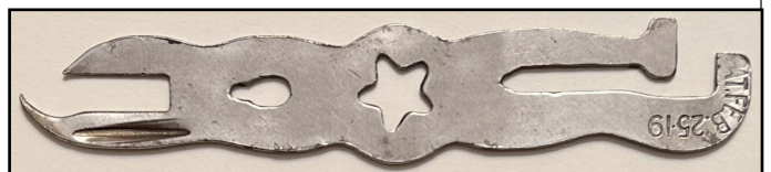
MIS-17 & 17A 3 3/4" Box Opener, Box Cover Prop, Nail Puller
