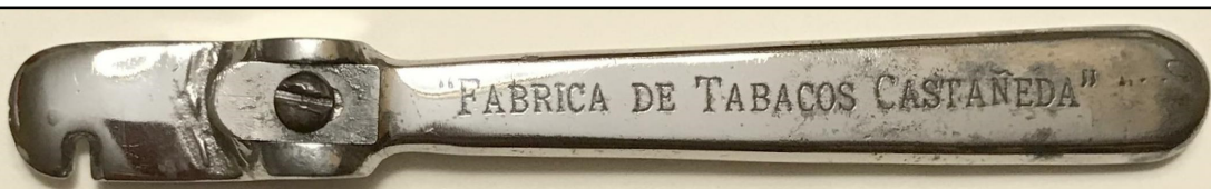
DHM-36 5 1/8" Notched Blade, Guide Along Double Hammers to Prevent Blade From Entering to Far Into Cigar Box, Flat Printing
