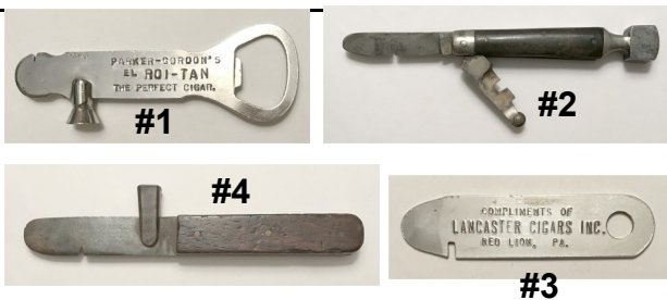
Figure 1. No. 1 — The most common cigar box opener. No. 2 — An early folding cigar box opener based on an 1868 patent. Also has a glass cutter. No. 3 — A late, very simple opener. No. 4 — A typical heavy-duty opener for com-
