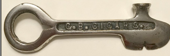
HKH-08 4" Notch, Hammer, Nail Puller at Ring End, Raised Printing in Bossed Area
