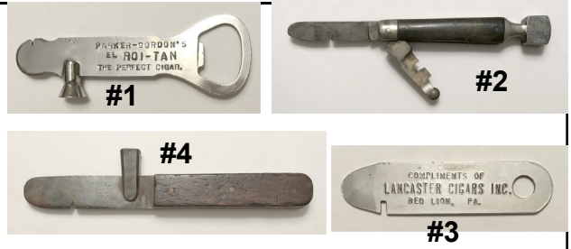
Figure 1. No. 1 — The most common cigar box opener. No. 2 — An early folding cigar box opener based on an 1868 patent. Also has a glass cutter. No. 3 — A late, very simple opener. No. 4 — A typical heavy-duty opener for commercial use.
