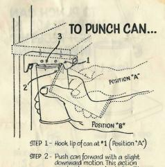
GTEP 2 - Push can forward with a slight downward motion. This action punches large pouring hole with punch marked \*2, and at the same time punching small vent hole with punch marked \*3
