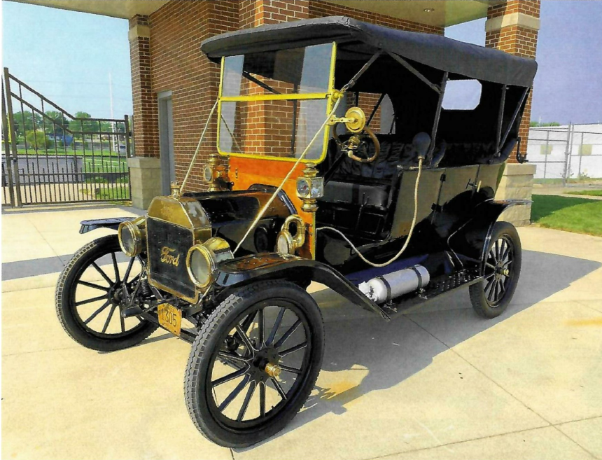
A Prest-O-Lite acetylene tank is located on the running board of this 1911 Model T Ford. This was the pre-electric light system, before batteries were used to power the headlights.
