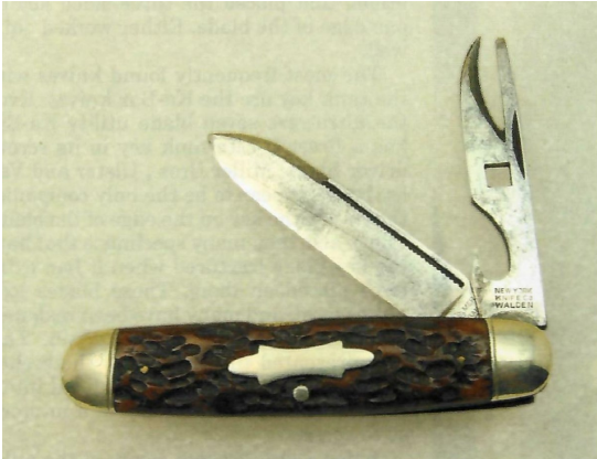
This is a two blade New York knife that features an unusual screwdriver with the Prest-O-Lite key. Another variation on a theme of specialty offered pocket tools.
