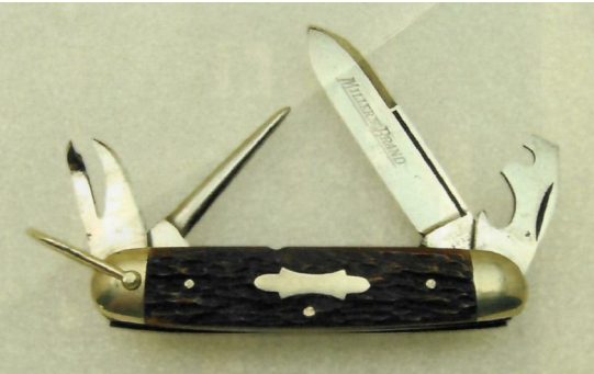
This unusual Miller Brothers utility knife also has the key wrench in its screwdriver blade.
