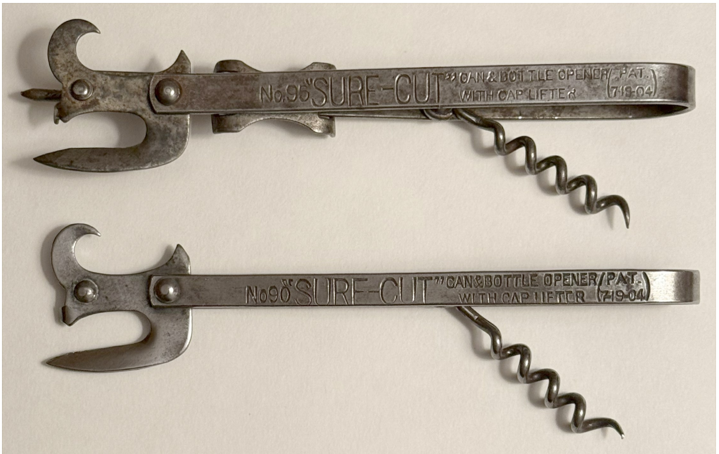
Two Sure-Cut steel handled Can Openers with a Corkscrew (Top: No. 95 sliding blade holder Bottom: No. 90 without sliding blade holder)
